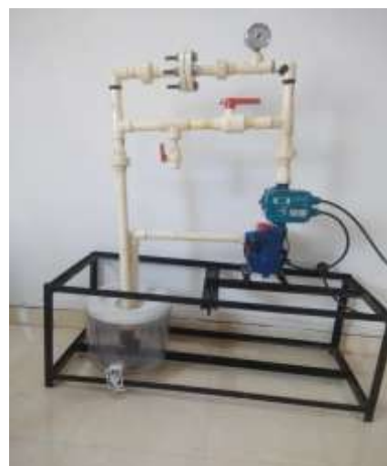
Fig.no.2. Setup of Hydrodynamic Cavitation Reactor
